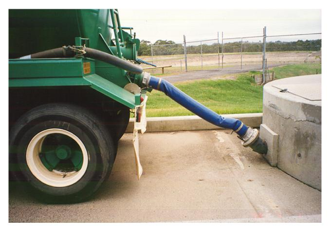
Figure 8. Tanker unloading effluent through flexible connection and KAM-LOK coupling
