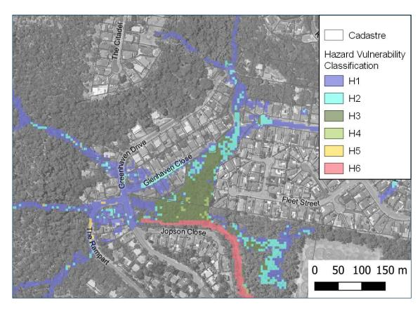
Figure 9.6 Flooding Hazard near Glenhaven Close - 1% AEP, 6 Hour Event
