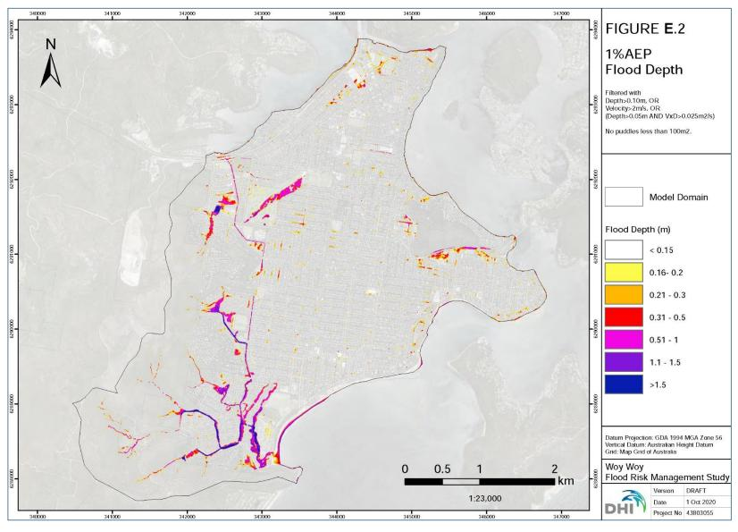
Figure 8.1 Peak 1% AEP Flood Depths
