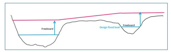
Figure 10.5 Flood Planning Level interpolated from two separate design flood levels
