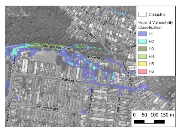
Figure 9.8 Flooding Hazard near Maitland Bay Drive - 1% AEP, 6 Hour Event
