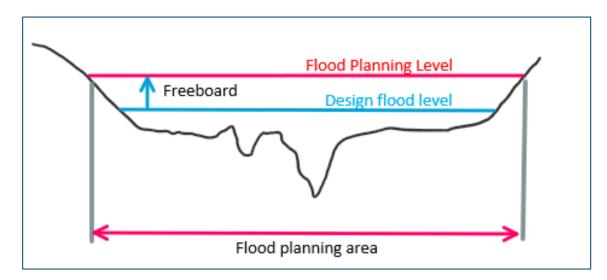
Figure 10.2 Traditional approach of defining Flood Planning Area by vertically raising the design flood level by a freeboard
