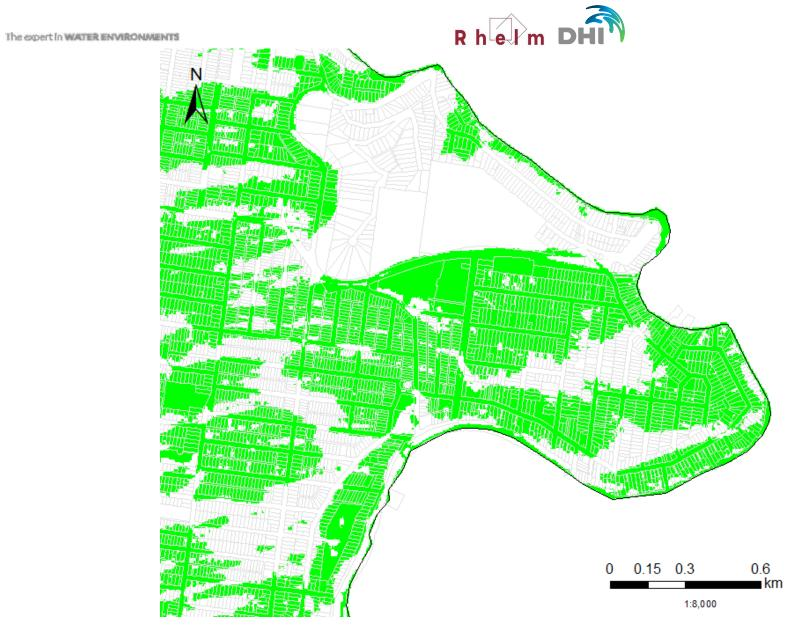
Figure 10.12 Flood extent of 1%AEP design level plus 500mm freeboard in Booker Bay
