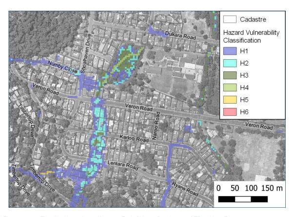
Figure 9.5 Flooding Hazard near Western End of Veron Road - 20% AEP, 1 Hour Event
