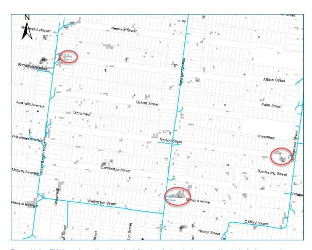
Figure 13.3 FM03 nominated locations for infiltration devices in the area with relatively deep sand layer
