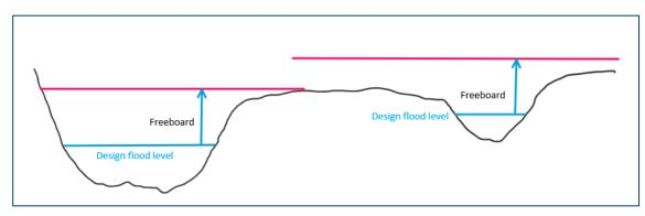
Figure 10.3 Different Flood Planning Level from two separate flood areas
