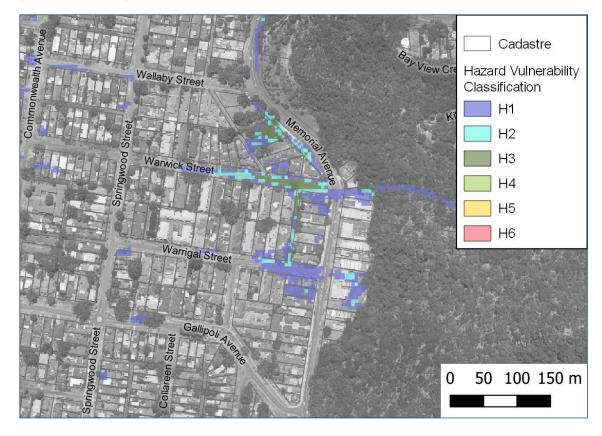
Figure 9.7 Flooding Hazard near Warwick Street - 1% AEP, 6 Hour Event
