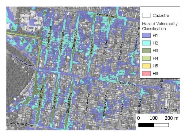
Figure 9.10 Flooding Hazard near Ryans Road – PMF, 2 Hour Event
