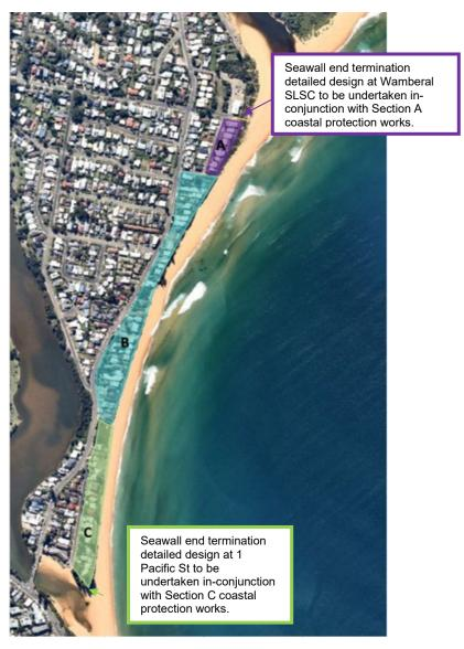
Figure 4.1: Divisions for staged seawall construction
